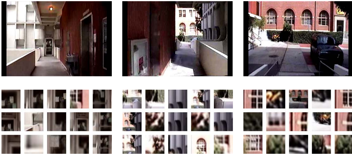
Figure 2. Top-level visual words selected during training for three of the five classifiers. Each visual word is represented by the average of the image regions corresponding to the SIFT features that build that visual word. A few of the selected visual words have negative weights (e.g., fourth visual word from top-left in the second environment).
