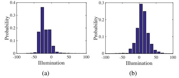
Fig. 4. Example of luminance of road pixels relative to mean image luminance. (a) Dry road. (b) Snow/ice-covered road.
